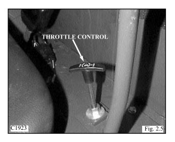
Before shutting off the engine, return the throttle control to idle position and allow the engine to cool at least 2 minutes.
