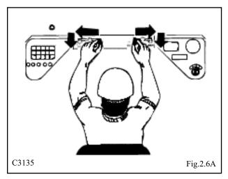
To operate the lift arm supports, first remove any bucket or attachment from the quick - tach; raise the lift arms to full height; push the two lift arm support pin handles, located directly in front of the operator at the top of the operator compartment (Fig. 2.6A), outward extending the lift arm locking pins (Fig. 2.6B). Slowly lower the lift arms down onto the pins. Always lift the lift arms off of the pins before retracting.
